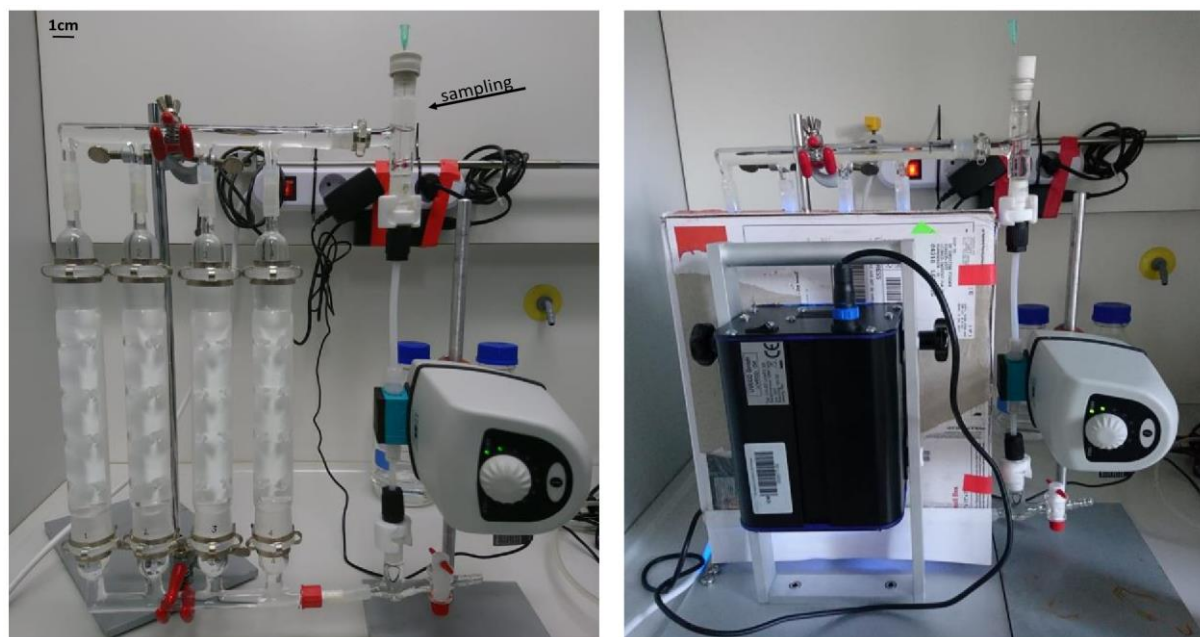
Fig. 1: Photographic images of the reactor, equipped with TiO 2 immobilized membranes within the glass tubes ( left ), and in operation with UV lamp and screen ( right ).
